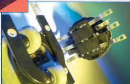
■ The "K" metering system is designed to provide an out-of-service storage position for the watt-hour meter allowing utilities to store the meter in the socket when it is taken out of service. This saves on remove/set orders and associated paperwork, and eliminates the need to bring the meter back to the meter shop and retest it before it goes back into service.
