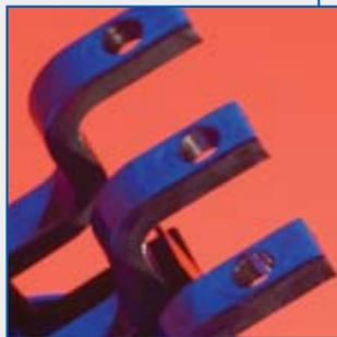
■ "K" mounting devices can be bypassed with manual bypass devices. The bypass clamps bridge from the line to the load bus and are capable of carrying 480 amperes continuously. The insulated handles on the bypasses prevent the enclosure cover from being installed with the bypass in place. Other types of bypasses are also available.
